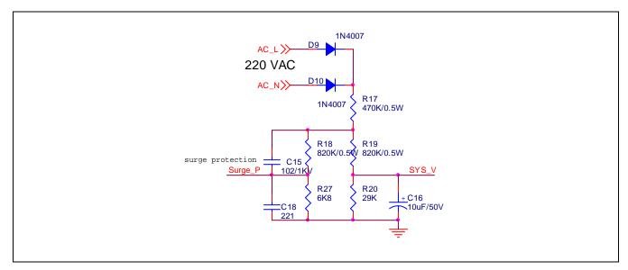
Figure 2-5 Voltage Measurement and Surge Protection Circuit
